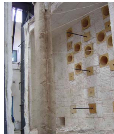
Structural Fire Test (Vertical Furnace)
