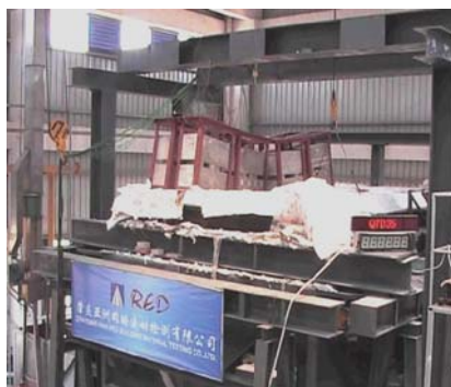
Structural Fire Test (Horizontal Furnace)
